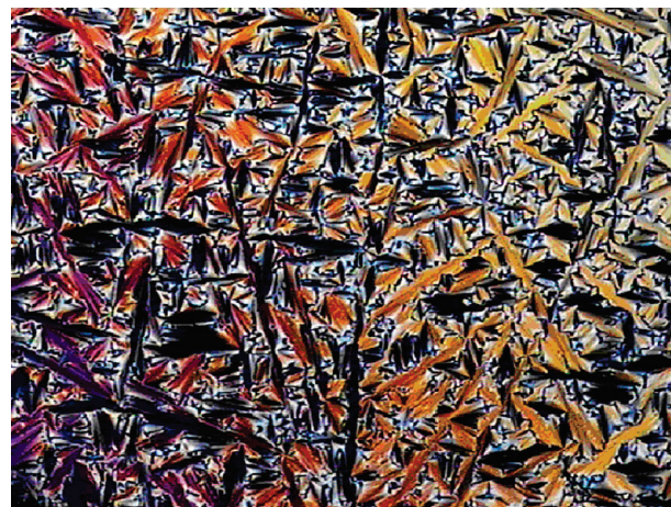
Figure 2. Optical polarizing micrograph of 6 on cooling. Magnification \times 33 ; T = 134\text{ °C} .
